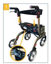
Place rollator on its wheels. Now press both side rails of the seat section downwards until they click into place. The rollator is unfolded correctly when the locking hook has clicked into place (pic. 1).
