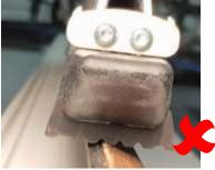
3. The Gripline ends of both sides of the ramp must rest firmly on the level surface.
