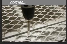
7. Use the pervading screw with associated nut and washer on the bottom.
