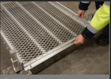
5. Mount the ramp attachment (KRL) in the slot at the lower part of the ramp (same when it
