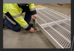
8. If desired adjust the foot end on the legs. Up to +50mm only.
