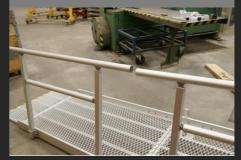
12. Mount the bottom and upper part of the handrail and tighten the screws.
